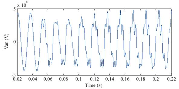
Fig. 2. Details of the voltage on phase a, transformer is energized at  $t = 0.05 s$ .
