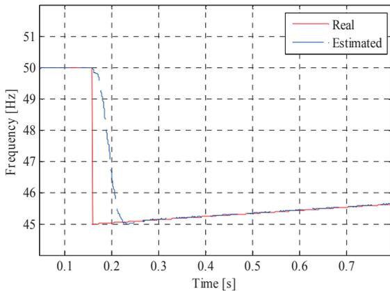
Fig. 5. Estimated frequency using UKF in a dynamic simulation.
