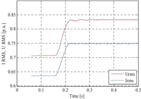
Fig. 4. Estimated RMS using UKF in a dynamic simulation.
