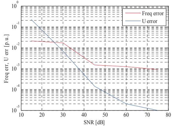
Fig. 1. Maximum amplitude and frequency errors vs. signal to noise ratio with constant initial covariance.
