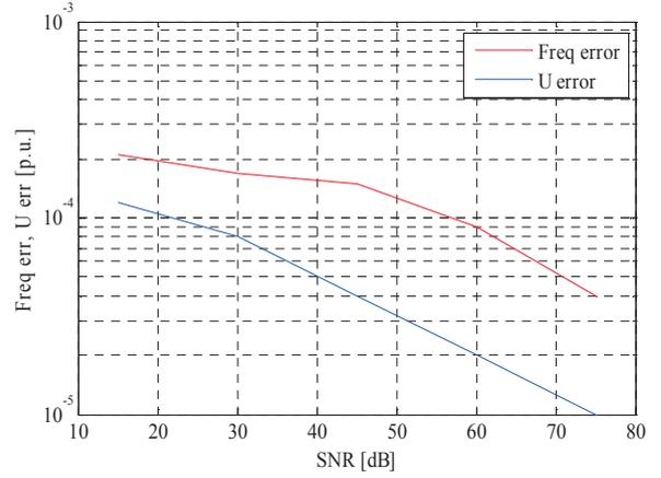
Fig. 2. Maximum amplitude and frequency errors vs. signal to noise ratio with adjusted initial covariance.
