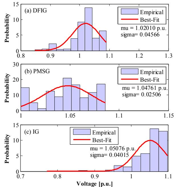
Fig. 8. PDF of the terminal voltage for the considered WT.
