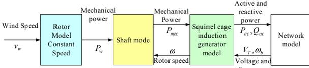
Fig. 2. General structure of tems FSWT using SCIG including the subsets and their interactions [16].
