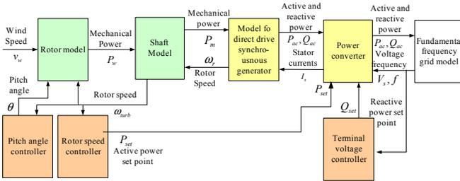
Fig. 4. General structure of typical VSWT using SG including the subsets and their interactions [1].
