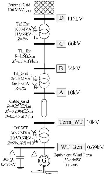
Fig. 6. Single-line diagram for the representative test system. Data of all components is depicted in the diagram. Qc: variable reactive power compensation.
