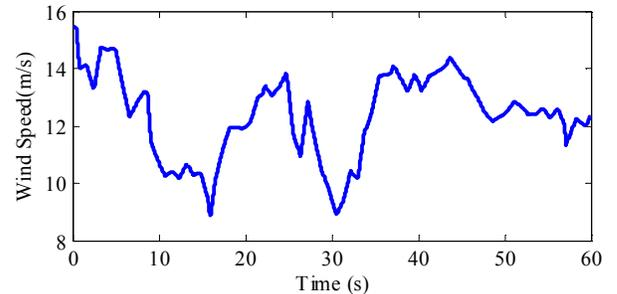
Fig. 5. Wind speed ( $v_w = 12.5258$  m/s mean value) time series used in the simulation [17].
