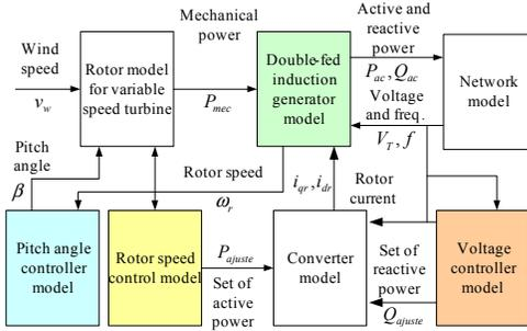
Fig. 3. General structure of tems VSWT using DFIG including the subsets and their interactions [1].
