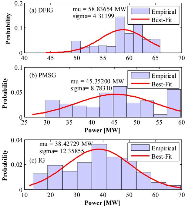
Fig. 8. PDF of the active power output for the considered WT.
